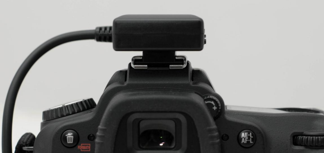
Diagram 1 : di-GPS® Mini 3L was mounted on the flash accessory shoe
