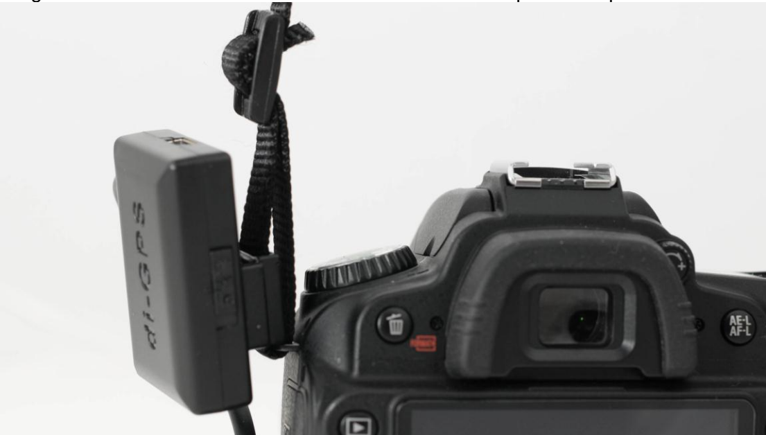
Diagram 2 : di-GPS® Mini 3L attached to the camera strap with strap mount accessory
